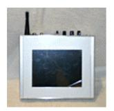
The RV 2400 is a combined portable receiver and monitor designed for setting up microwave links or use in remote surveillance operations.
