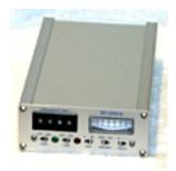
The RV 2000A is a receiver operating in the frequency band from 950MHz to 2050MHz. It is adjustable on the front panel by preset switches at intervals of 1MHz. The frequency range may be extended from 2051MHz to 2700MHz with a converter.
